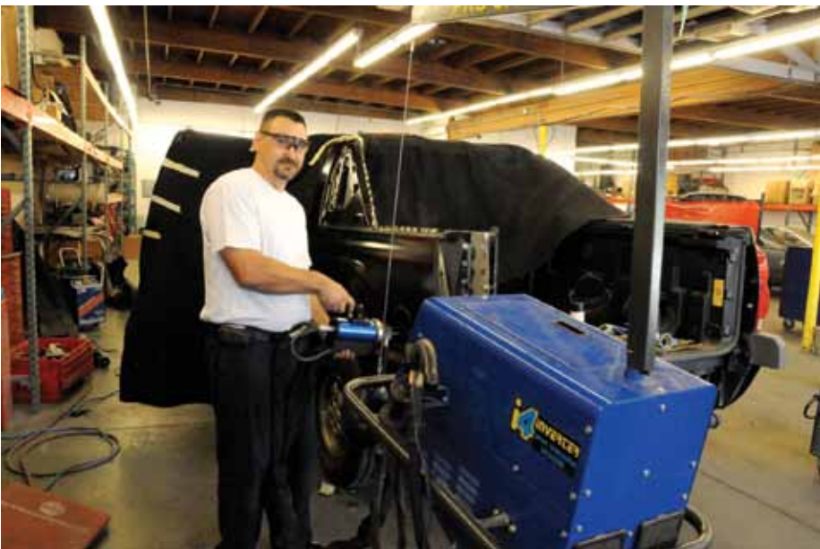
Body Technician Eugene Dorozhin uses G&R Body and Paints’ new state of the art spot welding system to prep a truck for painting.
